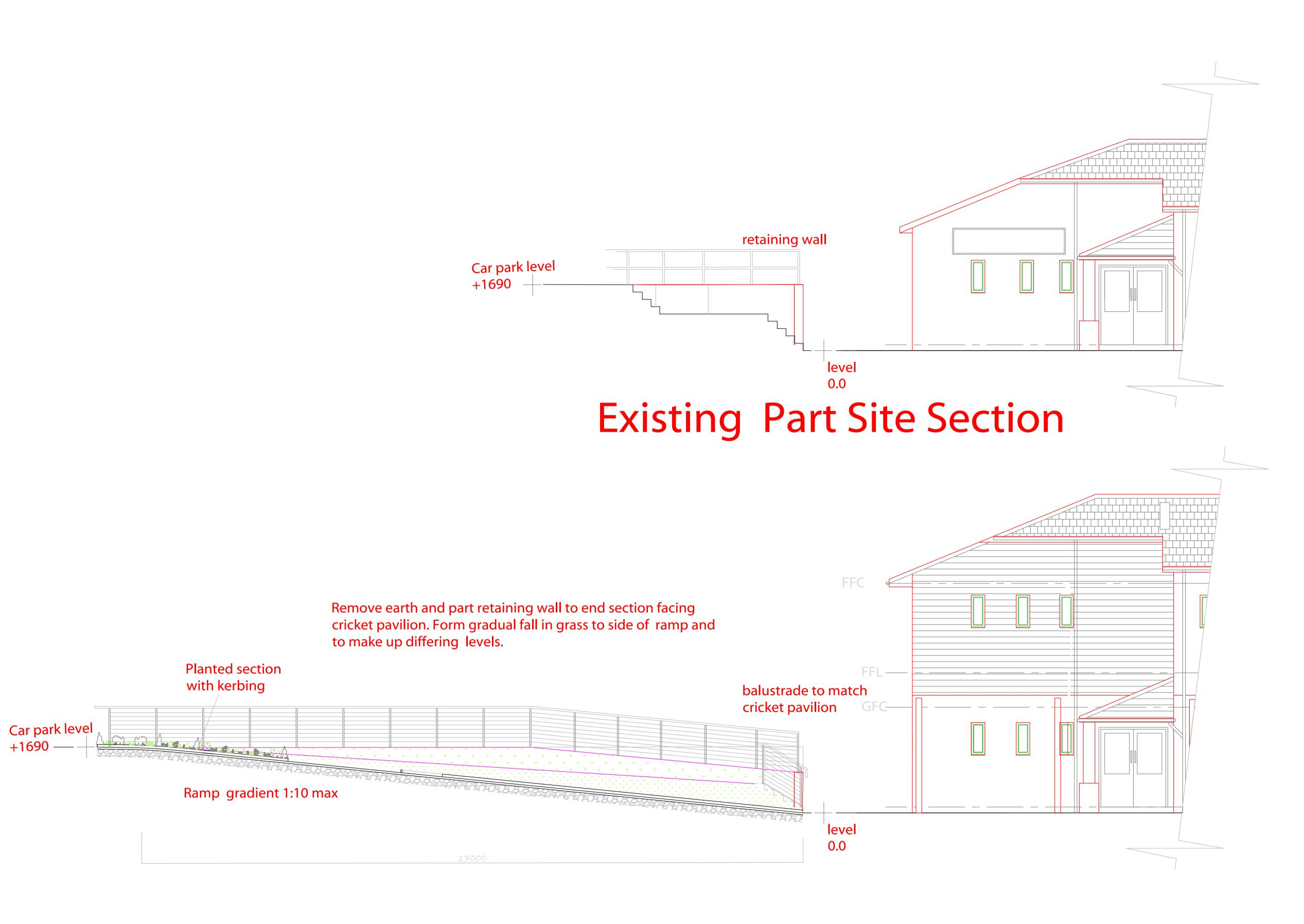
Proposed Site Section thru ramp
